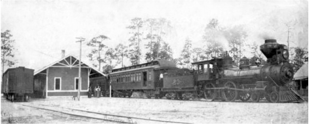
Jacksonville & Southwestern Railroad Company engine #23 at Newberry, Florida. It is an 1887 American 4-4-0 built by Baldwin Locomotive Works. W. H. Sealey is the man in the white shirt. Florida Photographic Collection.
