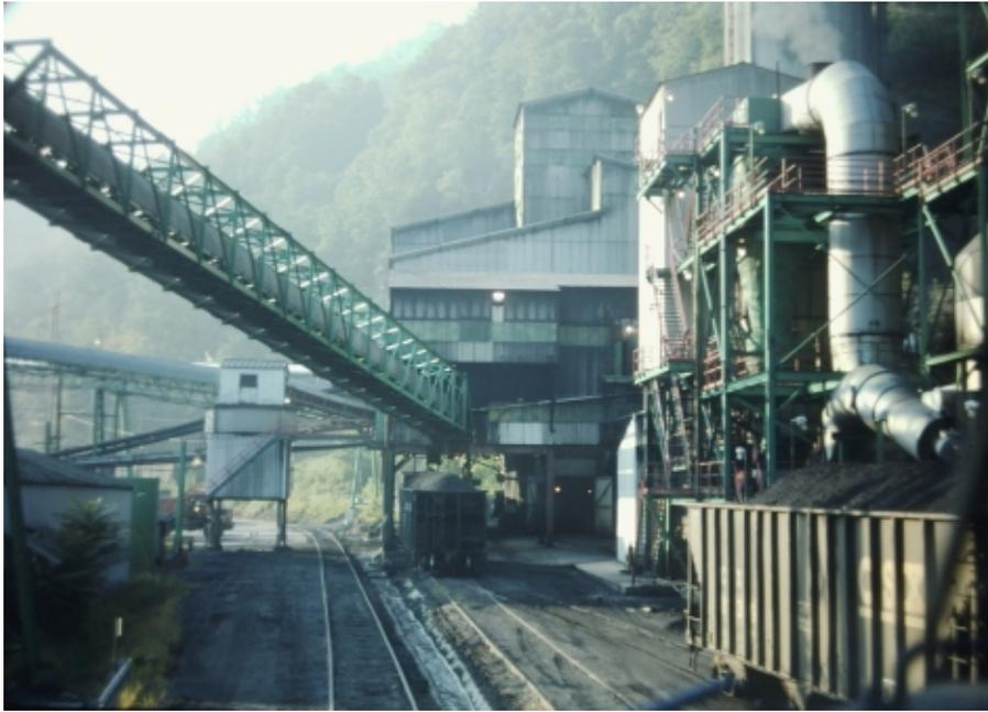
**Prenter Mine - on the right are coal cars that have just been loaded. Under the tippel are two cars being loaded. Soon the management coal rider will roll them down to the other coal cars. When the loaded track is full they'll start using the empty track. When we first arrived and pushed empties up to the three track yard, we shoved them through the tippel on the track in front of our engine.**
